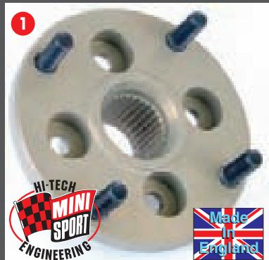
Designed and developed to be as strong and light as possible by our State of the Art Engineering Department on the latest Cad-Cam computers.
