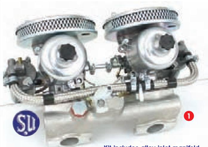
Kit includes alloy inlet manifold, linkages, fuel pipes, pancake air filters, needles and springs.
