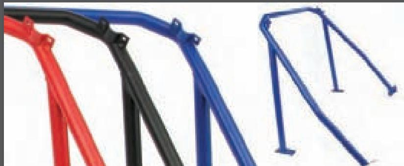
Mini Sport roll cages are produced to the highest standards using cold drawn steel tubing. These cages are for road use only and are available in three colours for the front and rear.
