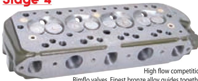
High flow competition Rimflo valves. Finest bronze alloy guides together with silicone chrome extra strong double valve springs. Compression ratio to suit application. Recommended for Rally/ Race.
